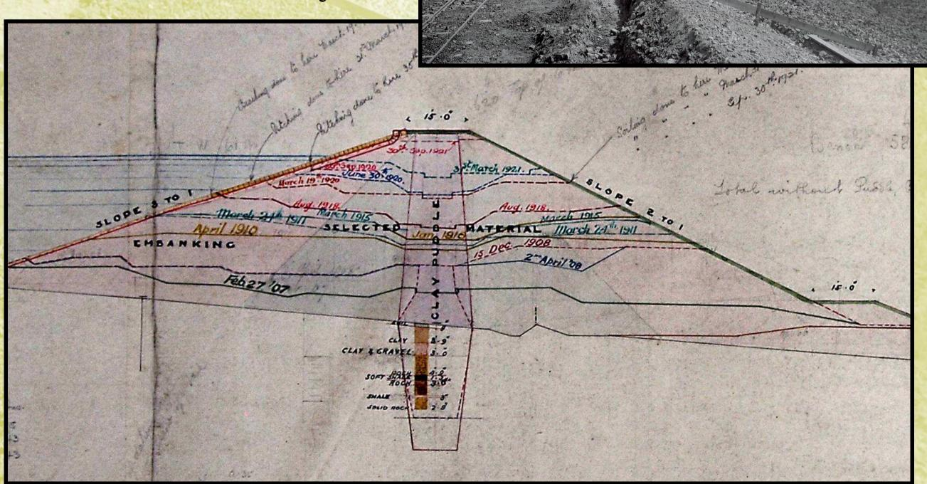
Drawing showing section of embankment - between Feb 27th 1907 and 30th Sept 1921.
